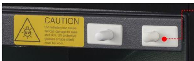
To override the UV Safety interlock, pull the right hand door switch and then follow the on-screen instructions.
